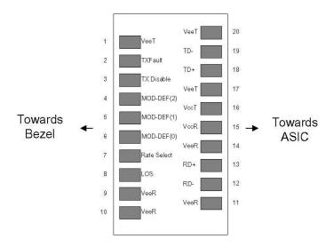
**Pin-out of Connector Block on Host Board**
